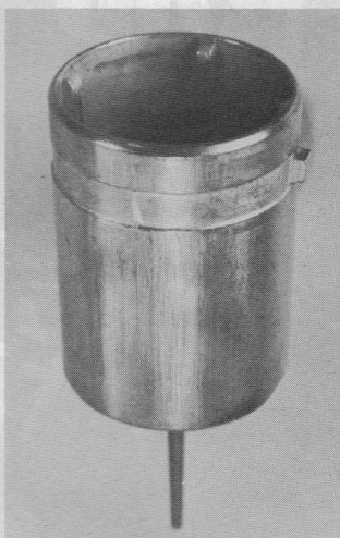
This Bing carburetor slide shows a fair amount of wear after 6000 miles. It makes carburetion a bit imprecise.
